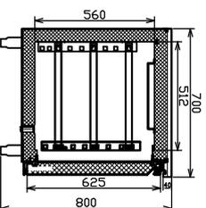
A: Please Follow the instructions, properly install the water supply tube and drain tube for the equipment, and reserving additional space of 10mm at the installation site to make the installation requirements. (Air cooling equipment needs more space to meet the air flow and heat discharge.)
